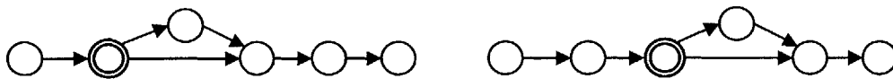
Figure 8-4: Two minimal representations of activity sequences \langle 1 \rangle, \langle 2 \rangle, \langle 3 \rangle and \langle 1 \rangle, \langle 2 \rangle, \langle 4 \rangle, \langle 2 \rangle, \langle 3 \rangle
