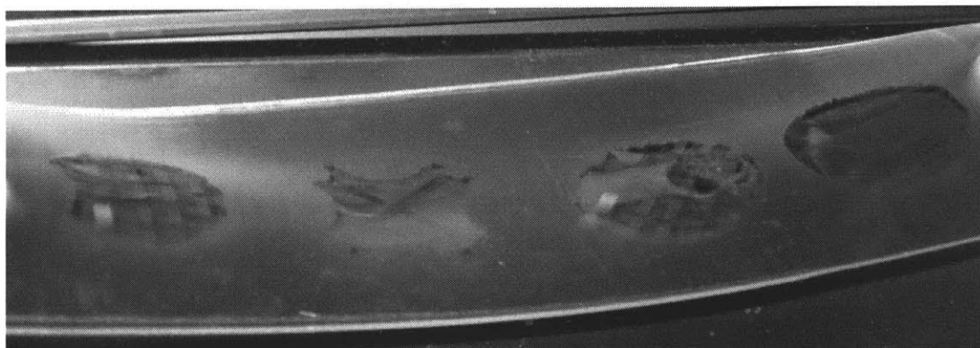
Figure 4.1.1C: Patterned PDMS sheet cured with four stamps placed in a line.
