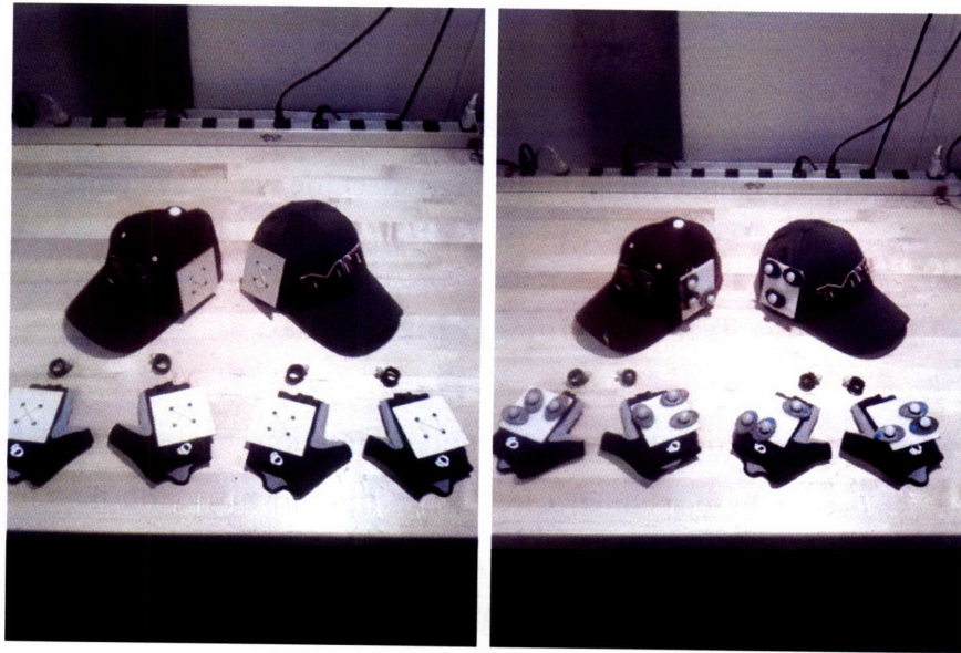
Figure 2-6: Hats, gloves, and rings outfitted with trackable markers.
