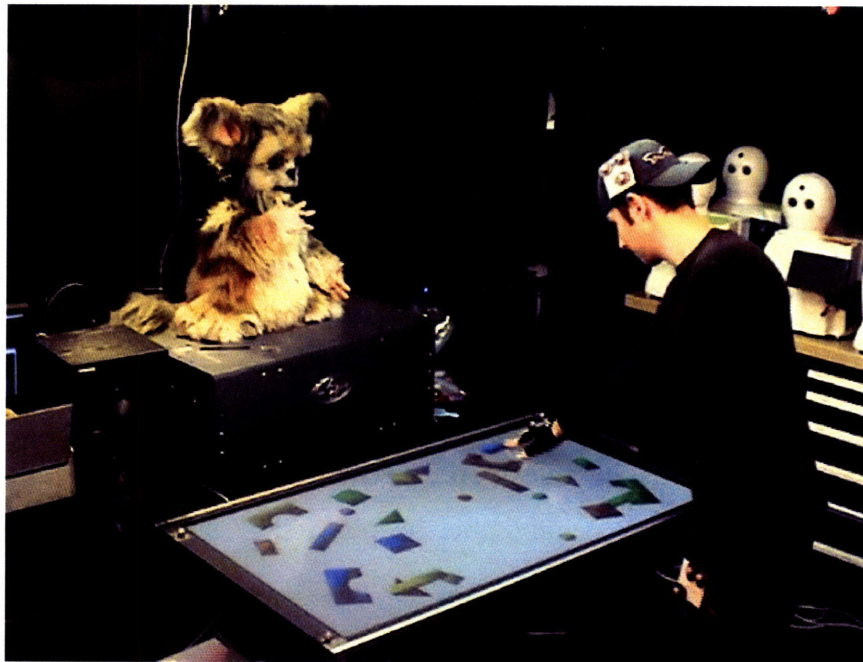
Figure 4-3: The robot took advantage of action timing and spatial scaffolding cues to learn through a live interaction with a human teacher.
