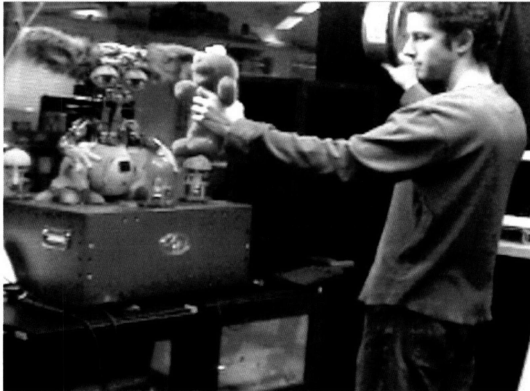
Figure 3-6: Leo in his workspace with a human partner. The human's attention on the toy influences the robot's attention as well as the referential focus.
