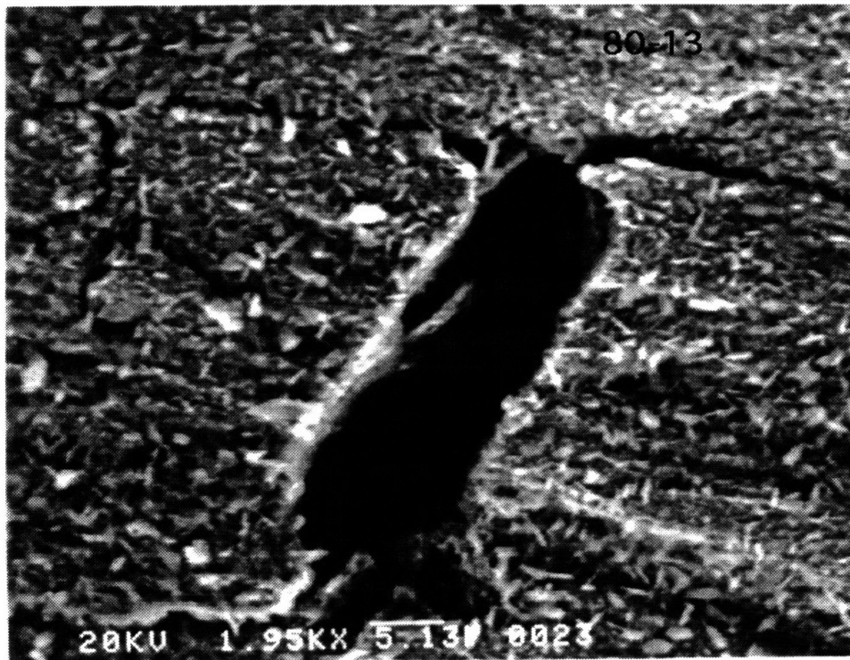
Figure 5-22. Side of specimen 80 (CP 304,AJ9139, 0.8 \times 10^{25} n/m 2 ) away from the fracture showing typical blunt crack (55 \mu m wide by 10 \mu m high).
