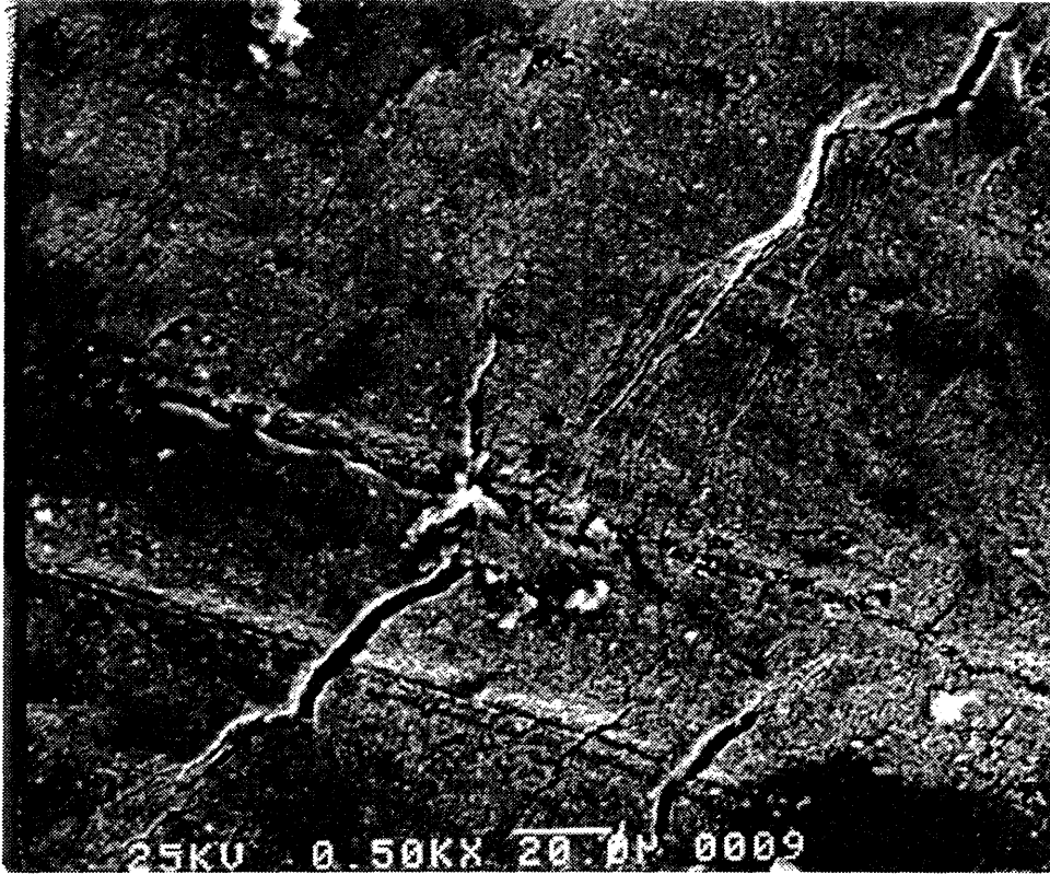
Figure 5-36. Side of specimen 82 (CP 304,AJ9139, 0.8 \times 10^{25} \text{ n/m}^2 ) away from fracture surface showing cracks with transgranular and intergranular modes.
