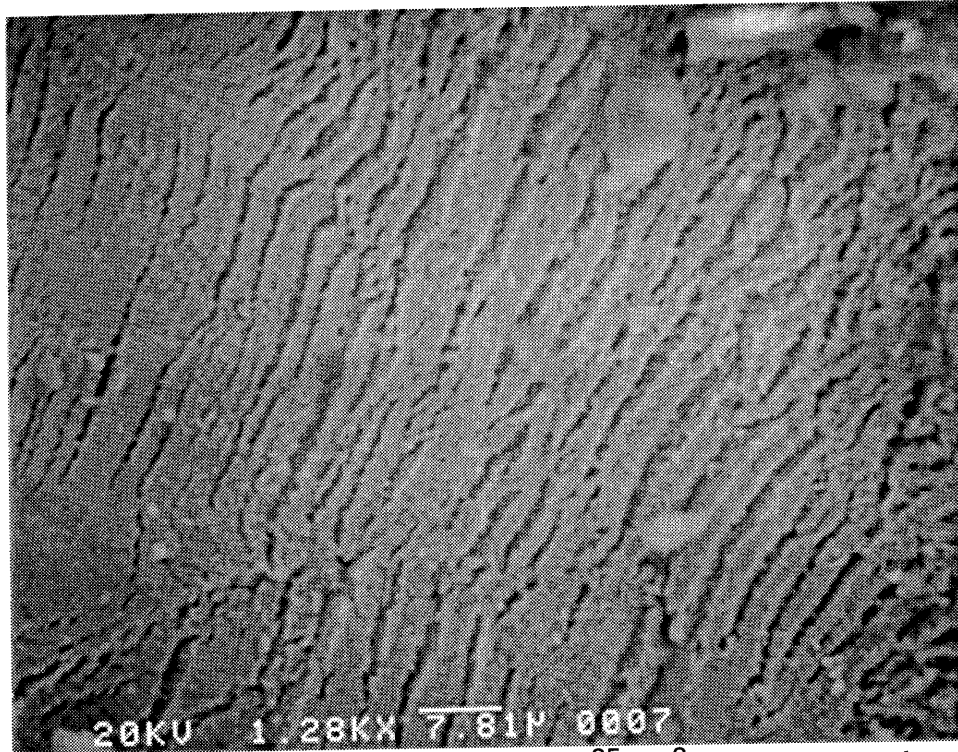
Figure 5-42. Side of specimen 11 (316L,K5, 0.74 \times 10^{25} \text{ n/m}^2 ) near fracture surface. Slip deformation appears uniform throughout cross section. Compare with localized regions of specimen 81 (CP 304, 0.8 \times 10^{25} \text{ n/m}^2 ) seen in Figure 5-29.
