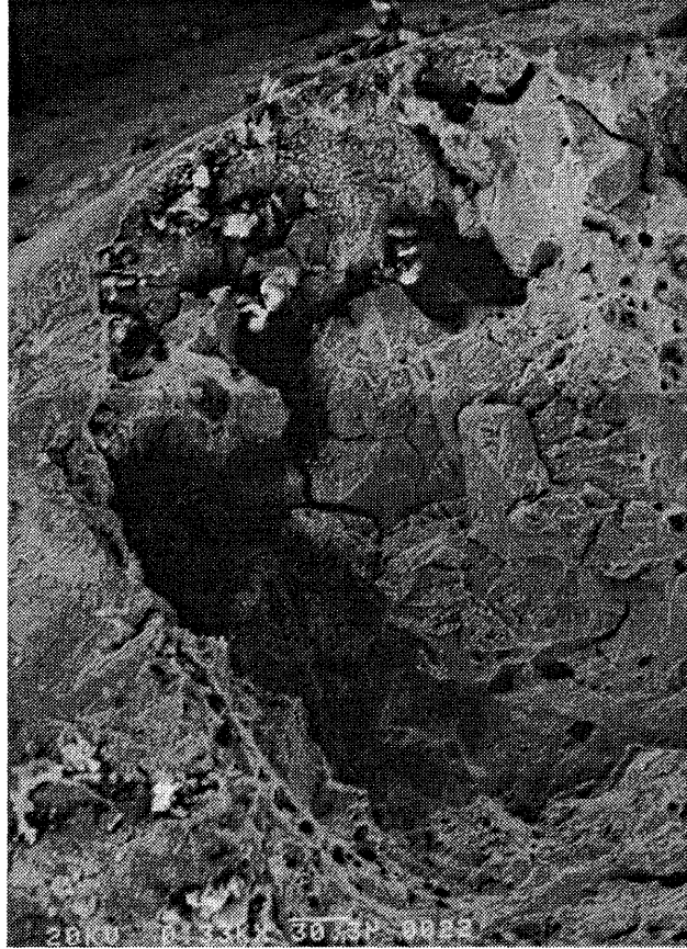
Figure 5-34. Upper intergranular region of Figure 5-32. Fracture surface near edge appears to begin in transgranular mode and changes to intergranular.
