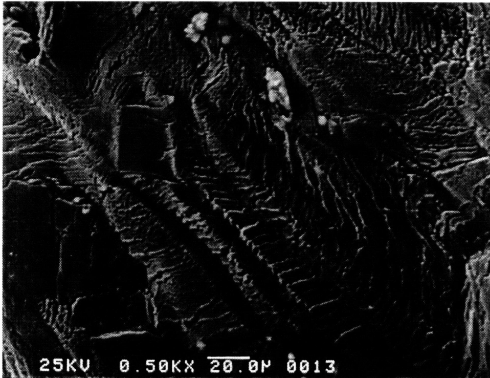
Figure 5-14. Side of specimen 98 (CP 304,AJ9139,0 n/m 2 ) away from the fracture surface depicting slip lines in regions. One region with lower density.
