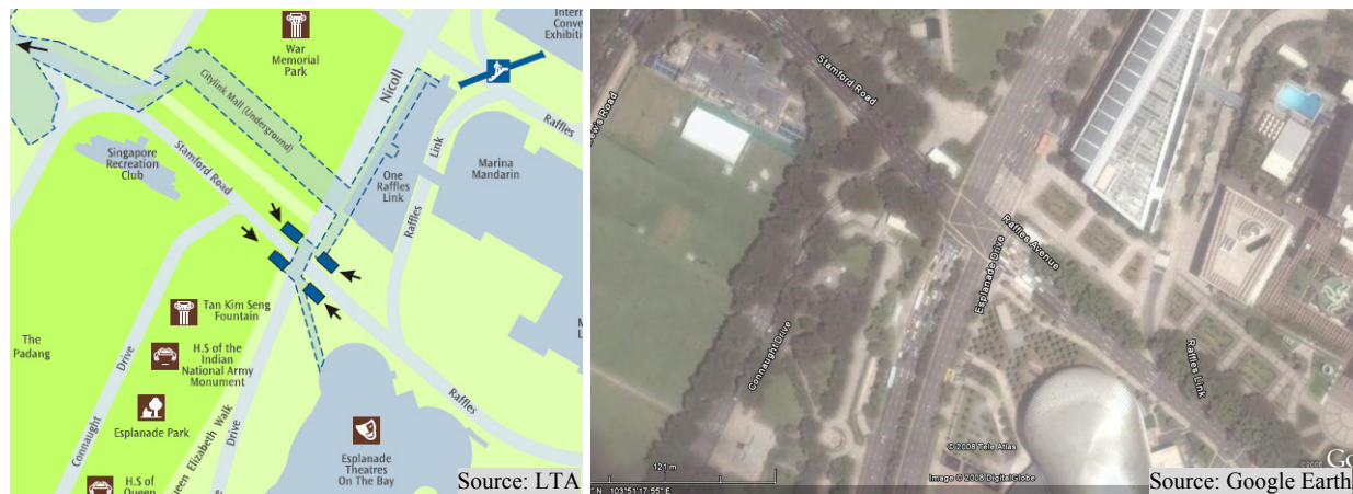
Fig 2.16 An example of an intersection in Singapore which restricts walkability
