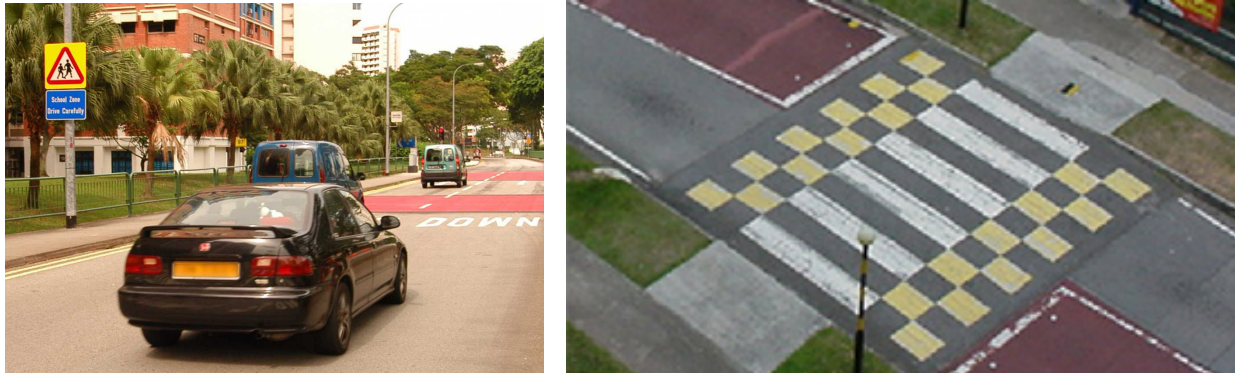
Fig 4.8 Typical traffic calming measures in the residential estates. Left- red texture pavement in school zones; right- raised pedestrian crossings (Source: LTA)
