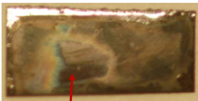
Figure 30. PVA-nitrate based YBCO film on buffered metal substrate, showing delamination
