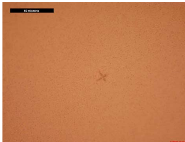
Figure 25. A PVA-nitrate film made from a 10 wt% PVA solution, showing small \text{Ba}(\text{NO}_3)_2 nuclei and one that had formed into a dendritic feature
