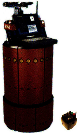
Figure 4-4: The B-21 Research robot (left) and the SwarmBot (right). The differences between the system parameters of these two robots produce very different robot speed ratios.
