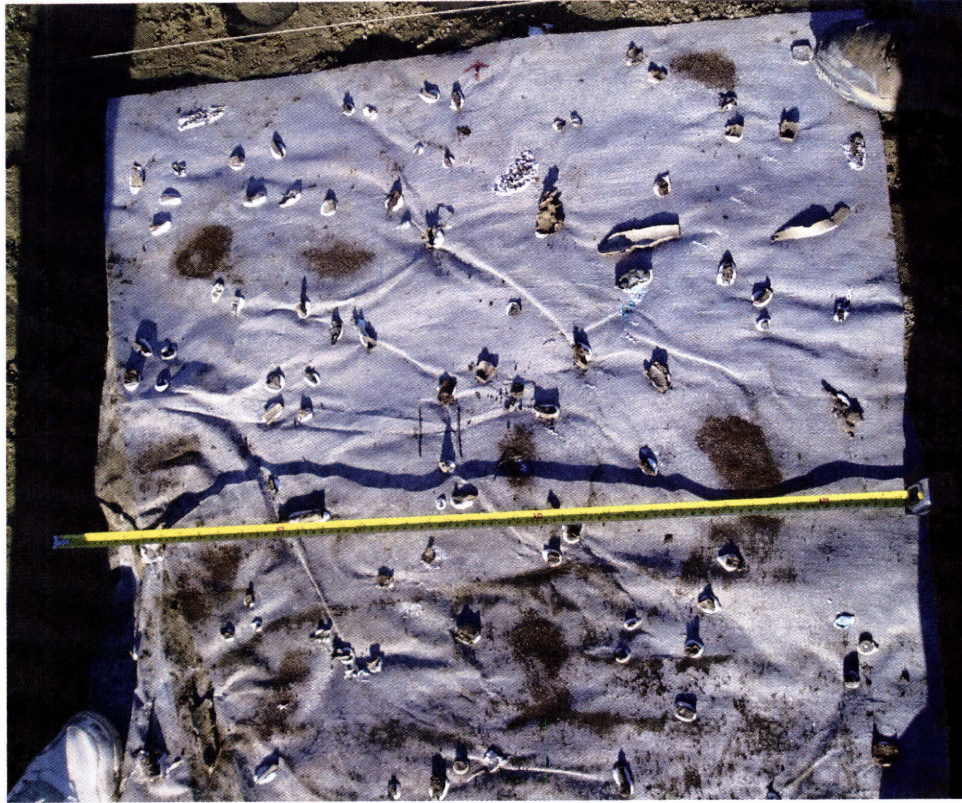
Figure 3-19: A mat of diffuse clutter pieces at a concentration seen at heavily contaminated UXO sites. Photograph courtesy of CRREL.
