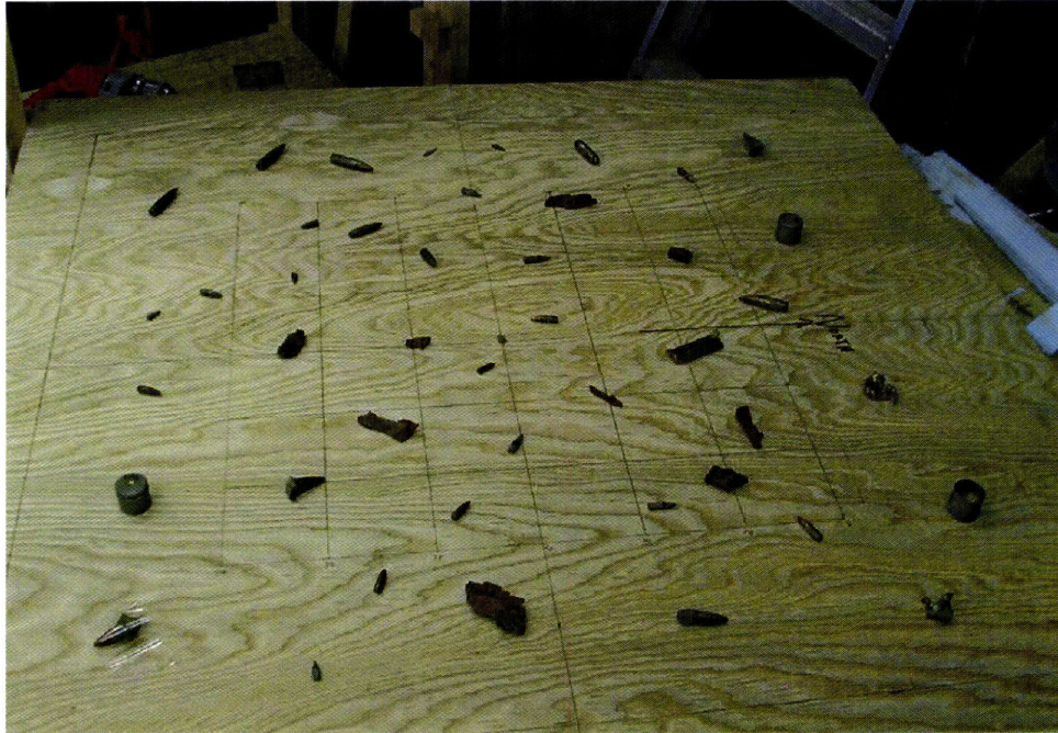
Figure 3-15: A mat of diffuse clutter pieces at a concentration deemed very significant for UXO contaminated land. This mat corresponds to the “full clutter” scenario. Photograph courtesy of CRREL.
