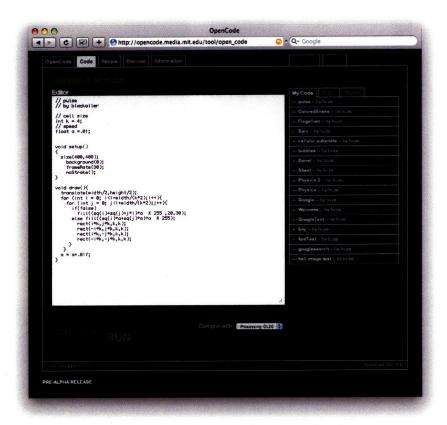
Figure 3-1: The main OpenCode programming interface, containing an editor window, and collection of links to scripts submitted by other users.
