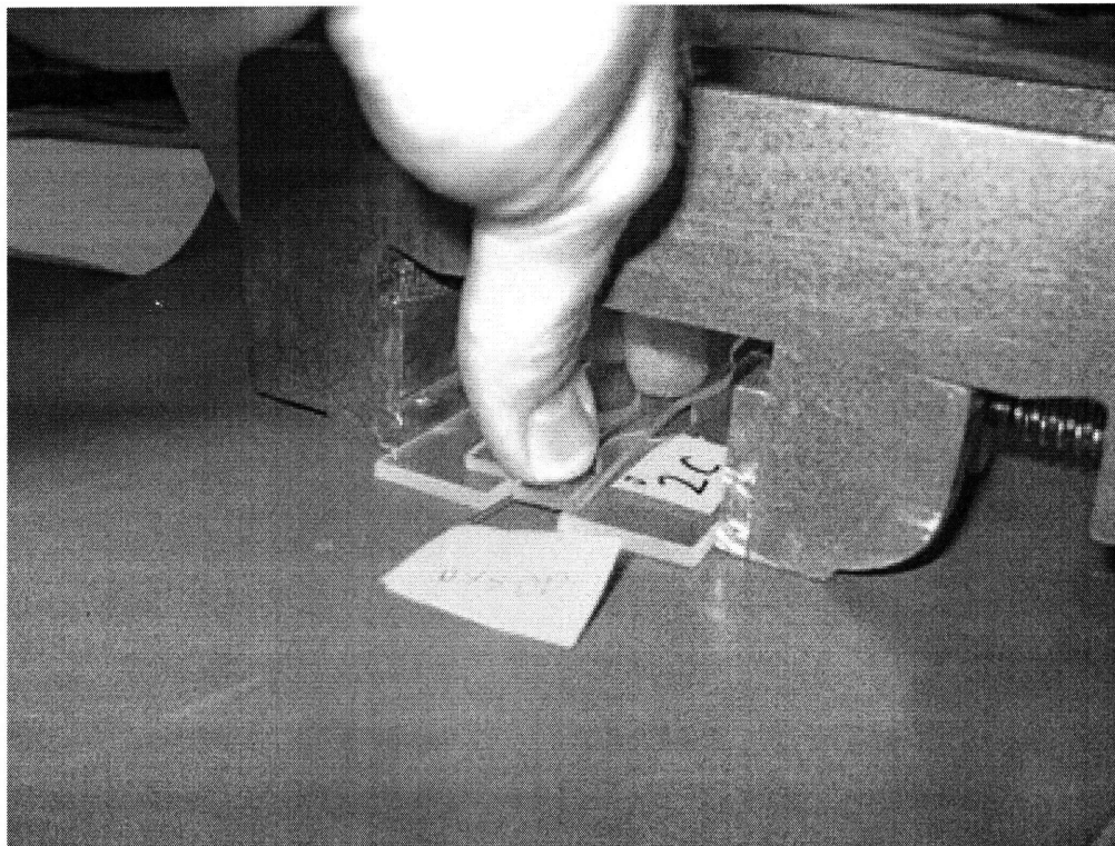
Figure 2-7: Tube and acrylic held down while being bent
