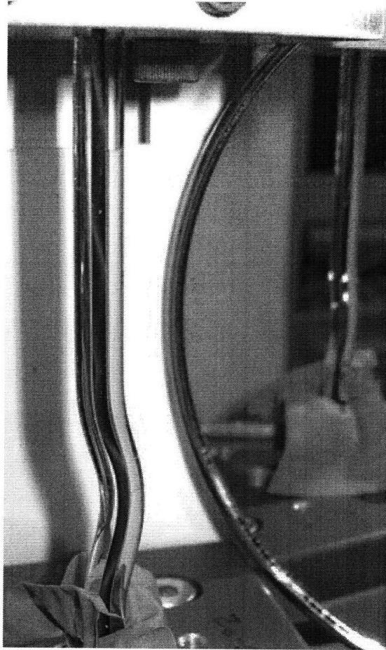
Figure 3-47: Helically buckled PTFE filament inside ink filled glass tube
