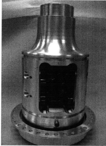
Figure 66: Differential Center Section with Gearing Installed and Left Eccentric and Bearing Pressed
