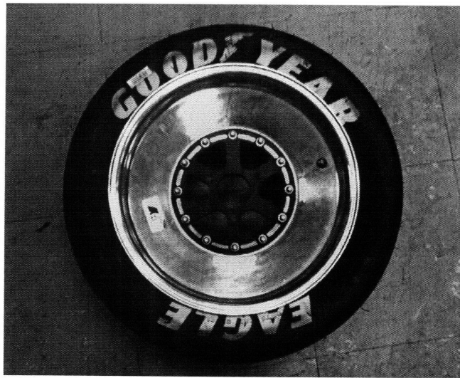
Figure 26: Completed wheel, featuring custom wheel center, Keizer wheel outer, and Goodyear Eagle Tire
