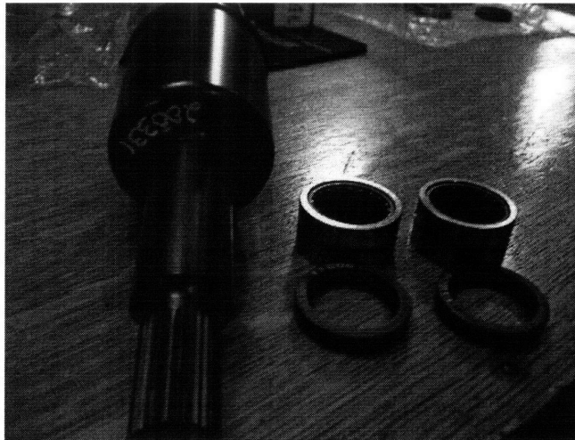
Figure 18: Inboard Stub-Shaft, Stub-Shaft Bearings, and Stub-Shaft Seals
