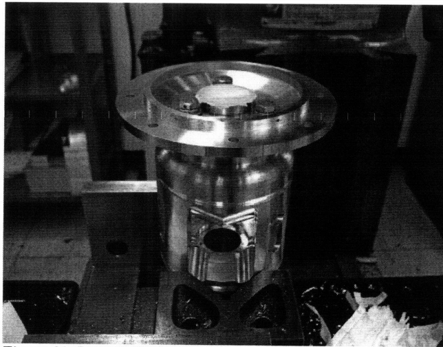
Figure 61: Input Bell Mounted to the Differential Center Section, Using Stub-Shaft Bearing to Ensure Concentricity
