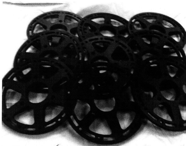
Figure 30: Wheel Centers after being Anodized in Black
