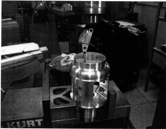
Figure 58: Differential Center Section Mounted in EZ-Trak Vise for Drilling Bolt and Pin Holes on Input Face
