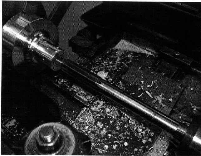
Figure 33: Reaming the Inner Bore of the Rear Hubs in Preparation for Splining
