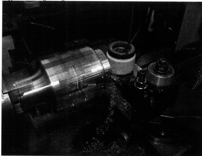
Figure 57: Finishing the Bearing Surfaces of the Differential Center Section
