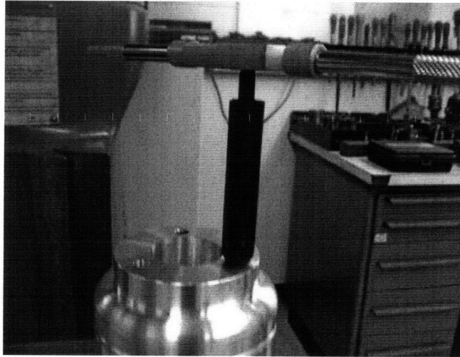
Figure 60: Installing the Helicoils on Input Face
