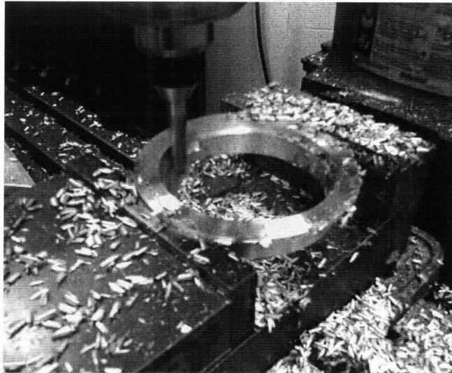
Figure 38: Milling the Inner Bore of the Left Eccentric, Using an EZ-Trak
