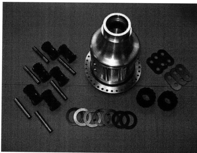
Figure 65: Differential Center Section with all Internal Components, including Gears, Washers, and Thrust Washers
