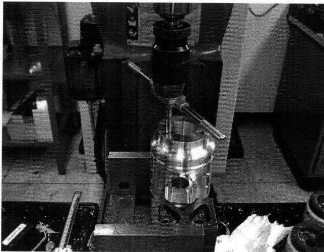
Figure 59: Tapping the Differential Center Section for Helicoils
