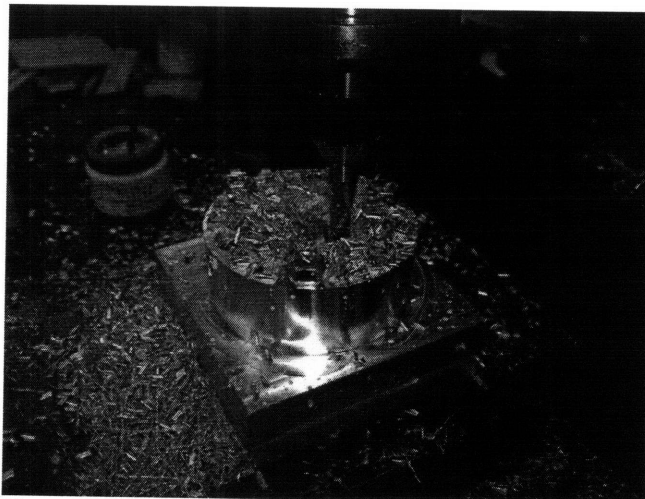
Figure 35: Cutting the Castle Nut Recess in the Rear Hubs using the Hub Jig Clamped in the EZ-Trak Vice
