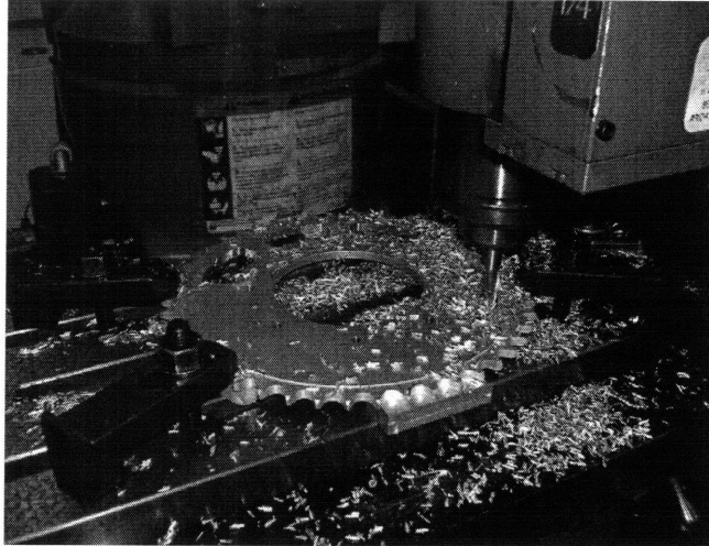
Figure 40: CNC Milling the Sprocket on an EZ-Trak
