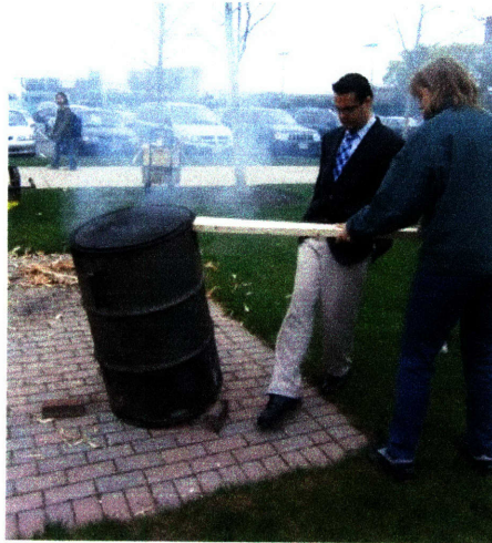
Figure A-6: Removing the stones from under the kiln
