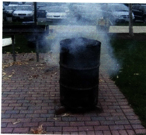
Figure A-5: Stifling the flame and sealing the kiln
