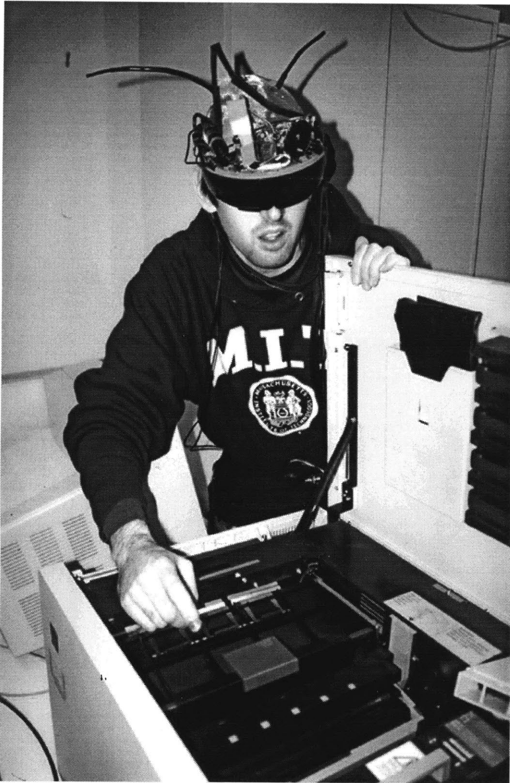
Figure 6-10: Equipment repair (in this case, a laser printer being serviced), in a 'mediated-reality' environment, using apparatus designed and built by author. Note the colored tape installed in the printer and on my fingertip, which is recognized by the camera in my eyeglasses.
