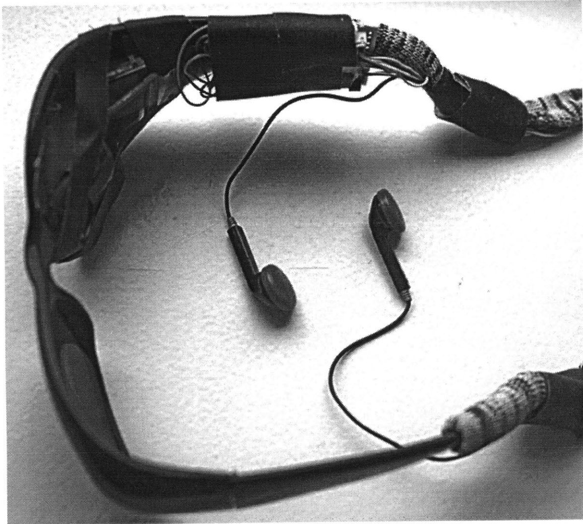
Figure D-20: Materials loosely held in place with gaffer's tape. All wiring is concealed in the "croakies" eyeglass safety strap. If earphones are desired, these are inserted now, and may later be stripped down for concealment into the glasses, or may be left as they are for less unobtrusive more conventional usage. Subsequently, the display unit, sensor array, and wiring is sealed in epoxy, consistent with the amount of space available between the head and the glasses. The unit pictured here is a right-eyed unit, while the original embodiments of WearComp7 were identical but left-eyed. Some variations were also two-eyed systems.
