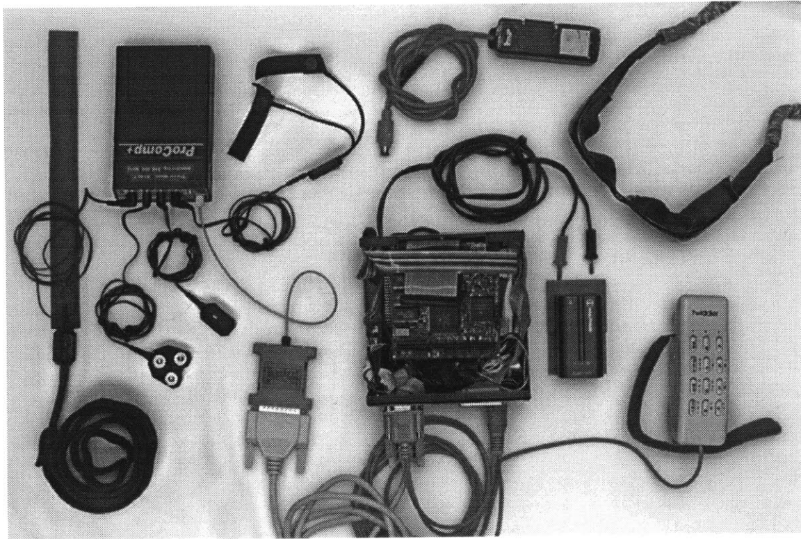
Figure 1-11: Personal Imaging workstation equipped with sensors for measuring biological signals. In the upper right are my "smart sunglasses" with built in video cameras and display system. These look like ordinary sunglasses when worn (wires are concealed inside the eyeglass holder). Immediately to the left of the glasses (top center of picture) is a commercial display unit called the Private Eye, which may be used instead of the "smart sunglasses" if imaging capability is not required. At the far left is an 8 channel analog to digital converter together with a collection of biological sensors, both manufactured by Thought Technologies Limited, of Canada. At the lower right is an input device called the "twiddler", manufactured by HandyKey, and to the left of that is a Sony Lithium Ion camcorder battery with custom-made battery holder. In the lower central area of the image is the computer, equipped with special-purpose video processing/video capture hardware (visible as the top stack on this stack of PC104 boards). To the left of the computer, is a serial to fiber-optic converter that provides communications to the 8 channel analog to digital converter over a fiber-optic link. Its purpose is primarily one of safety, to isolate high voltages used in the computer and peripherals (e.g. the 500 volts or so present in the smart sunglasses) from the biological sensors which are in close proximity, typically with very good connection, to the body of the wearer.
