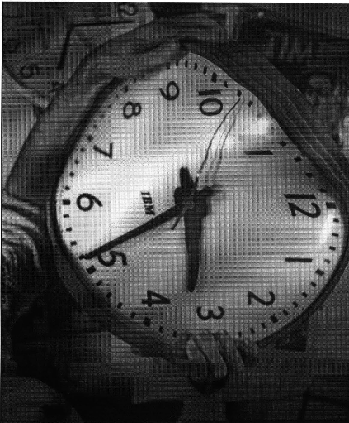
Figure 6-13: Twisted Time: An early embodiment of VibroTach was discovered while handling a clock into which I had built a radar system. I built the clock to tell distance rather than time, for an art installation in the 1980s. (The Doppler spectrum was effectively integrated with a gain that resulted in 1 minute of clock advancement for each 12 inches of distance, thus carrying the clock 60 feet down a long corridor advanced it approximately 1 hour.) Most notably, a surreal experience resulted from handling the clock. The resulting synthetic synesthesia could best be described as a feeling as though there were strings attached to every object in the room, and that all those strings passed through the clockwork, so that in some sense, I could feel the movement of these objects at a distance. In this picture, I have attempted to convey the surreal effect of holding onto this special clock, through the use of an oblique slice in a spatiotemporal volume. (c) Steve Mann, 1989.
