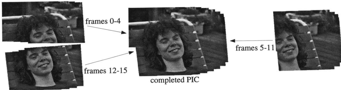
Figure 4-14: Subcomposites are each made from subsets of the images that share high quantities of mutual support and low estimates of mutual error, and then combined to form the final composite. (PIC stands for Pencigraphic Image Composite.)
