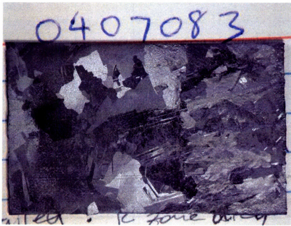
Figure 4: Samples recrystallized under the harsh profile, after texture etching. The furnace failed when sample 0407083 was only partway through, so only the right half is recrystallized. The successfully recrystallized half was still used as a data point.
