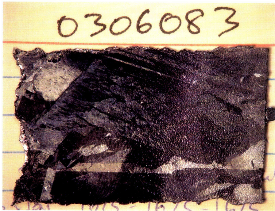
Figure 2: Typical grain structure after recrystallization and texture etching. Above is a top view of a sample, and below is a bottom view of the same sample, rotated about its long axis. Grains are millimeters to centimeters in length, with elongation down the pull direction of the sample and at a shallow angle ( 30^\circ to the pull direction). The differences in surface finish obscure some grains, but most features are still visible.
