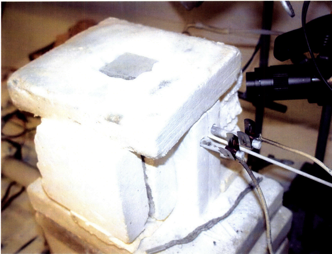
Figure 13: Aperture furnace used for insulation testing. The material under test sits in the port in the furnace lid. The heater elements are IsquaredR's Starbar silicon carbide heaters. A type R thermocouple is used for temperature feedback.
