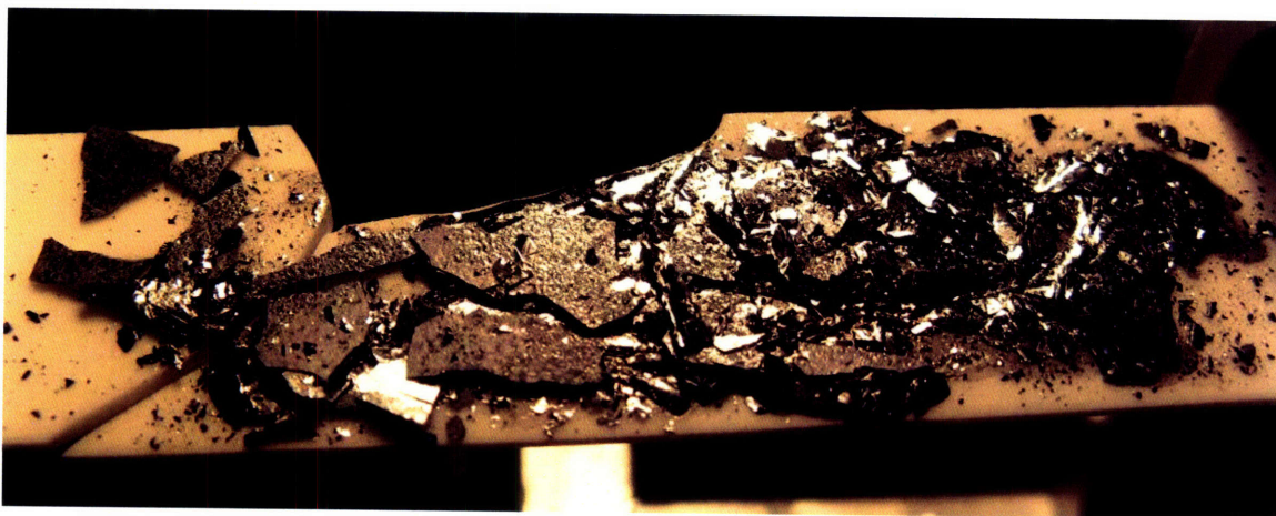
Figure 7: The remains of a wafer and alumina backing plate, after recrystallization without a separate release layer. Thermal stress from CTE mismatch was sufficient to break both the wafer and backing plate.
