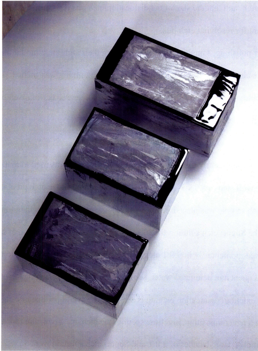
Figure 4: Samples mounted to aluminum blocks with wax, before grinding and polishing.
