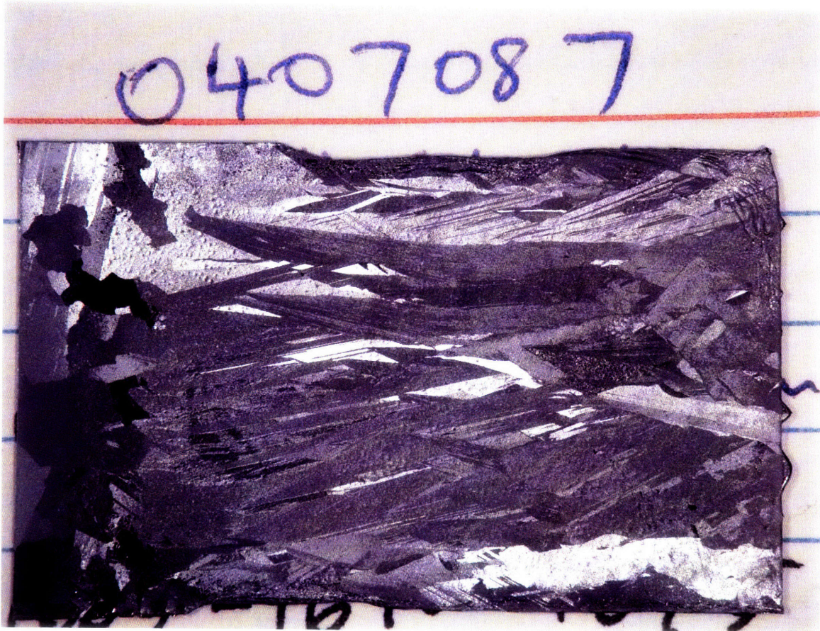
Figure 15: Camera image of a texture-etched sample, in which the heater power was lost most of the way through. The sample was being recrystallized under a gentle temperature profile. Recrystallized material is on the right; unrecrystallized material is on the left. Differences in principal dimensions of the grains are apparent.
