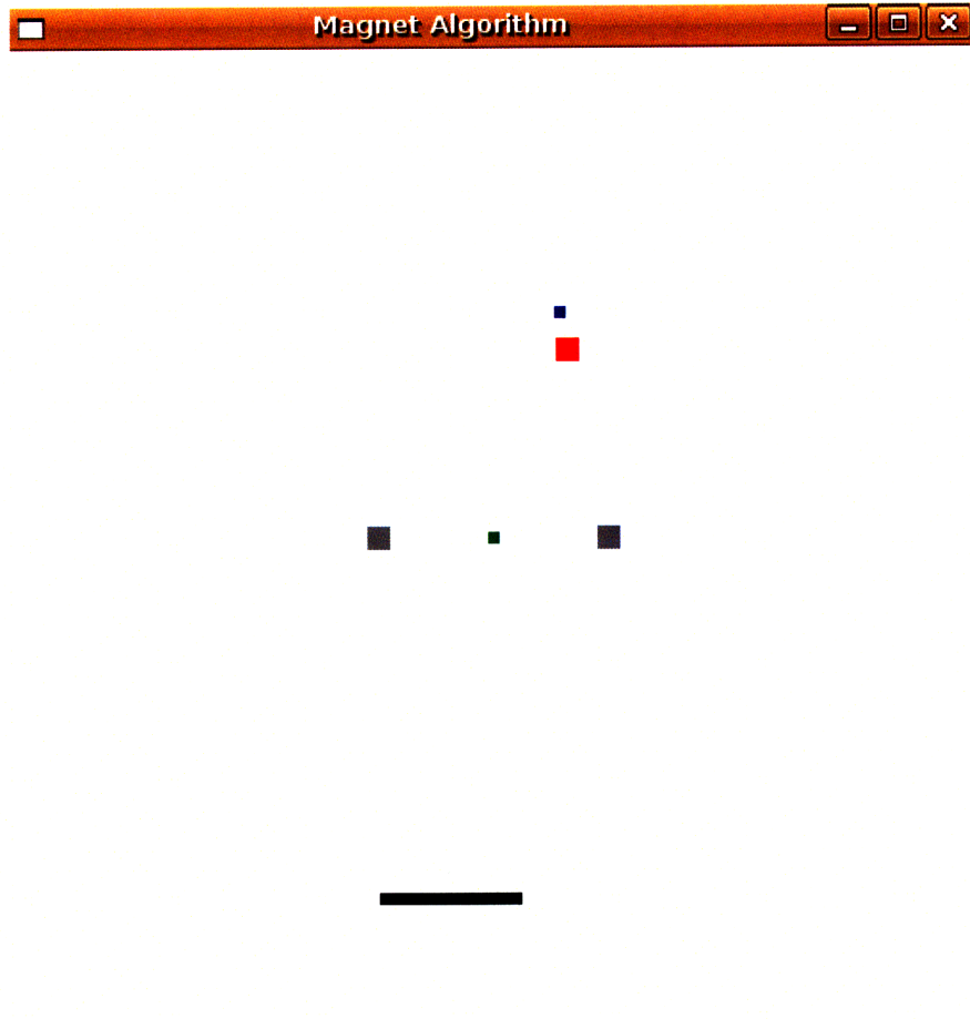
Figure A-2: Visual output of magnet simulation. Large box indicates actual magnet position, small box north west of it indicates calculated magnet position; three horizontally colinear boxes are two Hall effect sensors and their midpoint.
