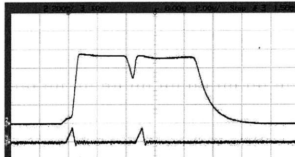
(a) Double pulsing with sleep timer set at about 4\mu\text{s}
