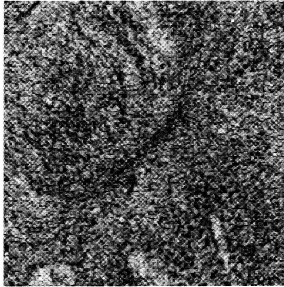
Figure 5-16: Weighting mask based on coherence map, (ERS-1 Data Set 1).
