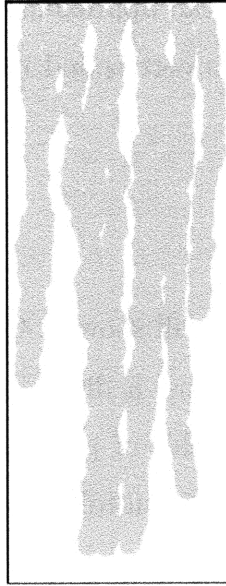
Figure 3-2: Area swept by the coverage-discs of 9 nodes that move according to the mobility model in an ideal-channel river with the simulation parameters described above.
