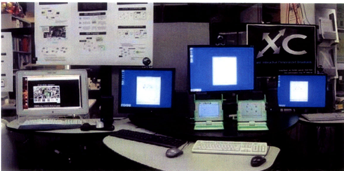
Figure 38. The second testbed of XCast system for sharing image and audio files: It consists of an event collection server and three wireless ad-hoc nodes.
