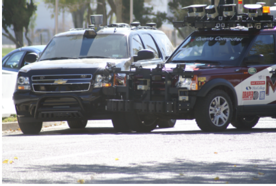
Fig. 1. Picture of the collision between MIT’s autonomous Land Rover LR3 ‘Talos’ and Team Cornell’s autonomous Chevrolet Tahoe ‘Skynet’ in the Darpa Grand Challenge 2007. It is known as the first well-documented collision between two full-size autonomous vehicles [4].
