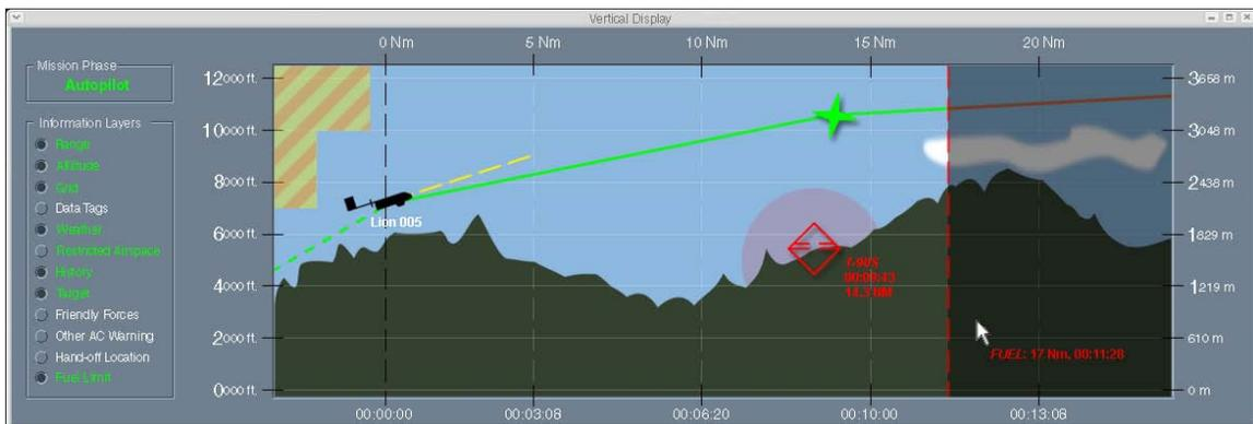
Figure 7 Vertical situation display with fuel limit layer
