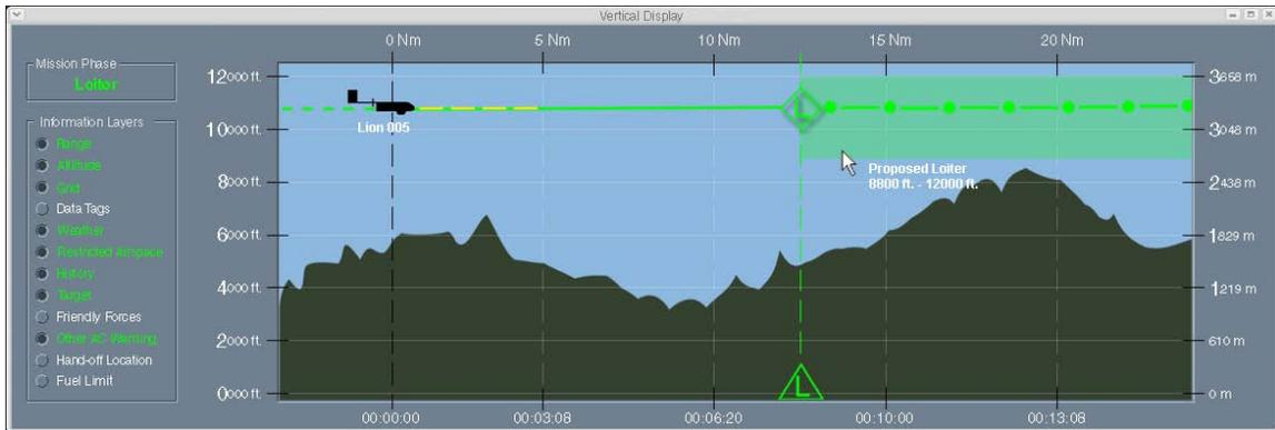
**Figure 13 Vertical display with proposed loiter pattern and permissible altitude range**
