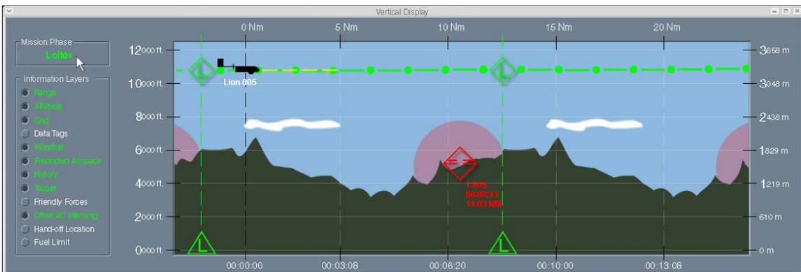
Figure 9 Vertical situation display, UAV in loiter pattern
