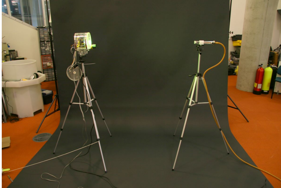
Figure 2-15: The flash output calibration test-bench. The flash is triggered in front of spectrometer’s cosine corrected optical probe. An optical fiber relays the light captured by the probe to the radiometric spectrometer. The black background prevents reflections from nearby objects from altering the measurements.
