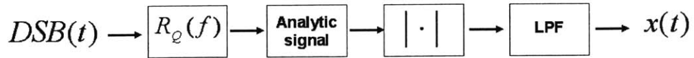
Figure F.7 Hilbert transform/low-pass filter method of envelope detection in a DSB signal. R_Q(f) is the frequency response of the quadrature filter that outputs the Hilbert transform of the input real signal. The complex analytic signal is then formed with its real part equal to DSB(t) and imaginary part equal to the Hilbert transform. Next, the magnitude of the analytic signal is taken. Finally, a low-pass filter acts on the signal.
