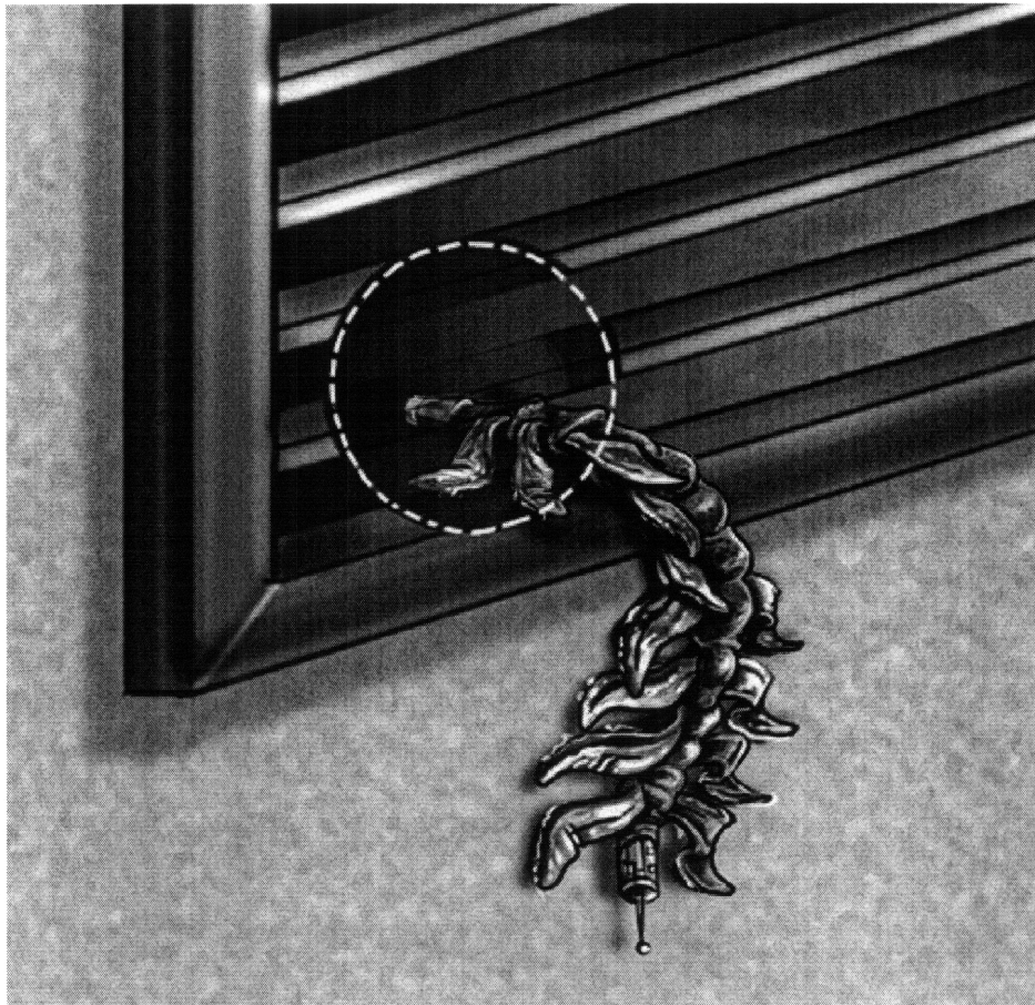
Figure 6-1: “Squishbot”, a proposed flexible robot capable of changing size and shape. Such a robot will use flexible actuators and apply a method of locomotion similar to robosnail 2. Squishbot a joint project between MIT and Boston Dynamics, and is funded by the Defense Sciences Office at DARPA as part of the Chembots program. Artwork is from Boston Dynamics [2]
