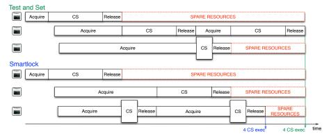
Fig. 1: The Impact of Lock Acquisition Scheduling on Asymmetric Multicores. Good scheduling finishes 4 critical sections sooner and creates more spare execution resources.
