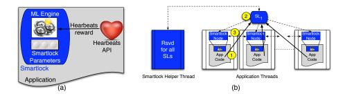
Fig. 3: a) Application-Smartlocks Interaction. Smartlock ML engine tunes Smartlock to maximize Heartbeat reward signal which encodes application's goals. b) Smartlock Implementation Architecture. Smartlock interface abstracts underlying distributed implementation and helper thread.
