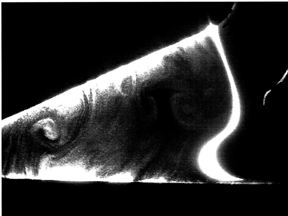
Figure 5-9: Near-bow streak videography at U=0.75\text{m/s} and x=27\text{cm} from waterline bow
