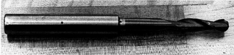
*Figure 7.13: Sleeve supported squeeze film prototype*
