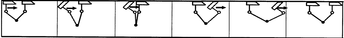
Figure 2-3: An illustration of the moonwalk gait. The planted foot is labeled in black while the moving foot is labeled in gray.
