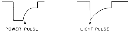
Fig. II-9. Comparison of transmitted power pulse and light pulse as a function of time.
