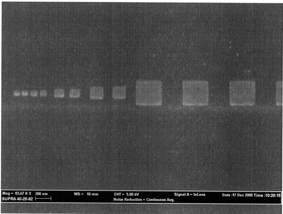
Figure 2-15. Electron beam lithographically patterned Ni catalyst dots, M=84K X.
