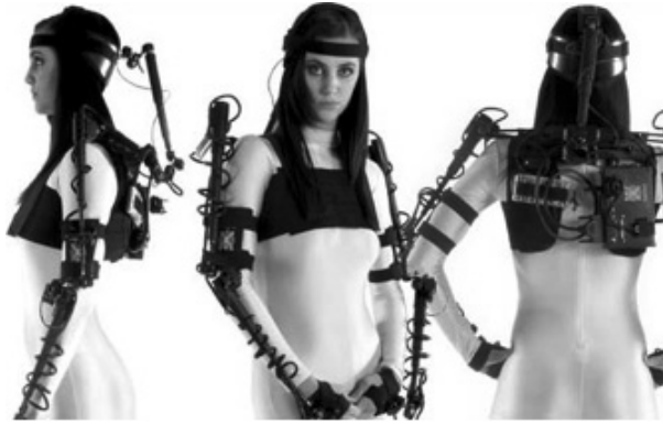
Figure 4: Meta Motion's Gypsy mechanical motion capture system
