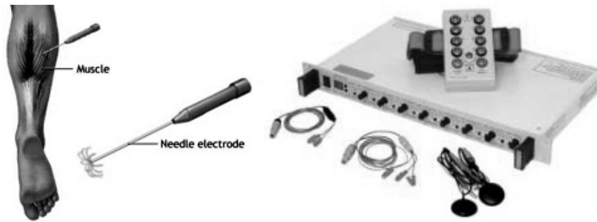
Figure 9: Invasive (left) and noninvasive (right) EMG systems (drbezner.com, www.health.utah.edu)
