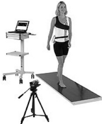
Figure 7: Force Plate for Gait Analysis (Noraxon U.S.A. Inc., 2009)
