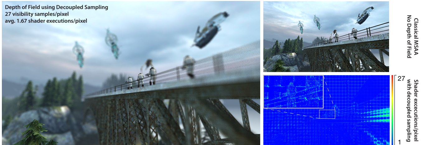
Fig. 1. Efficient depth-of-field using decoupled sampling in a recent Direct3D game, with 27 visibility samples per-pixel. The heat map encodes the amount of shading required over the image. Existing supersampling techniques would require 27 shading samples (red) over the entire image, which is prohibitively expensive, while decoupled sampling achieves similar quality with an overall average shading cost of only 1.67 samples per-pixel, similar to current edge multisampling antialiasing (MSAA) with no depth-of-field or motion blur. The visible tile structure in the heatmap is due to the rasterizer scanning pattern.
