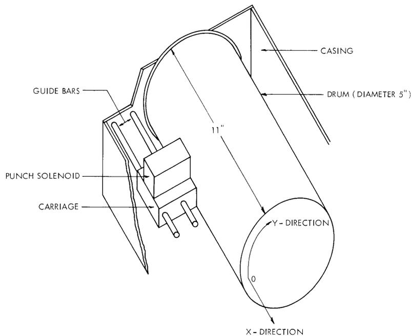
Fig. XII-14. Picture Brailer – mechanical transport and punch.
