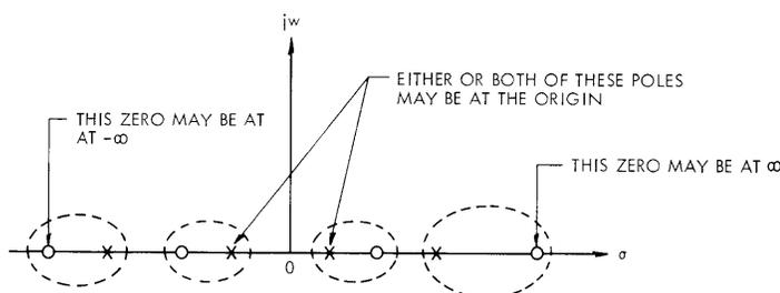
Fig. XII-8. Pole-zero plot of an R,  $\pm$ C driving-point impedance.
