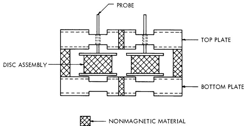
Fig. XII-13. Side view of the assembled device.
