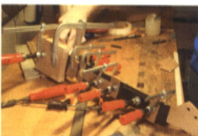
Fig. 124 Preparing the neck for the truss rod (left)
