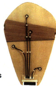
Fig. 67 Digital version's resonator, back side, with 4 piezoelectric sensors
