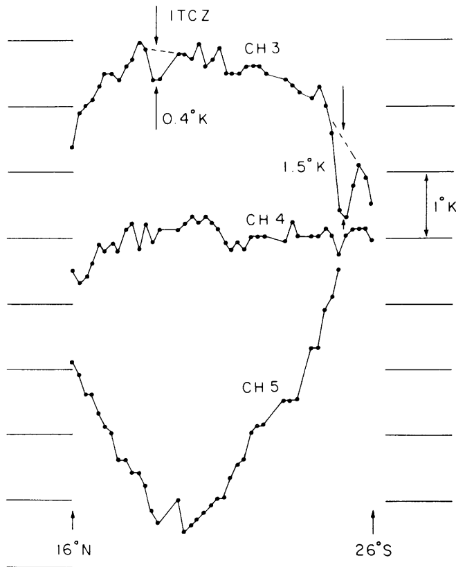
Fig. II-1. Relative brightness temperatures observed during orbit 163 as the satellite passed from 16° North to 26° South over the intertropical convergence zone (ITCZ).
