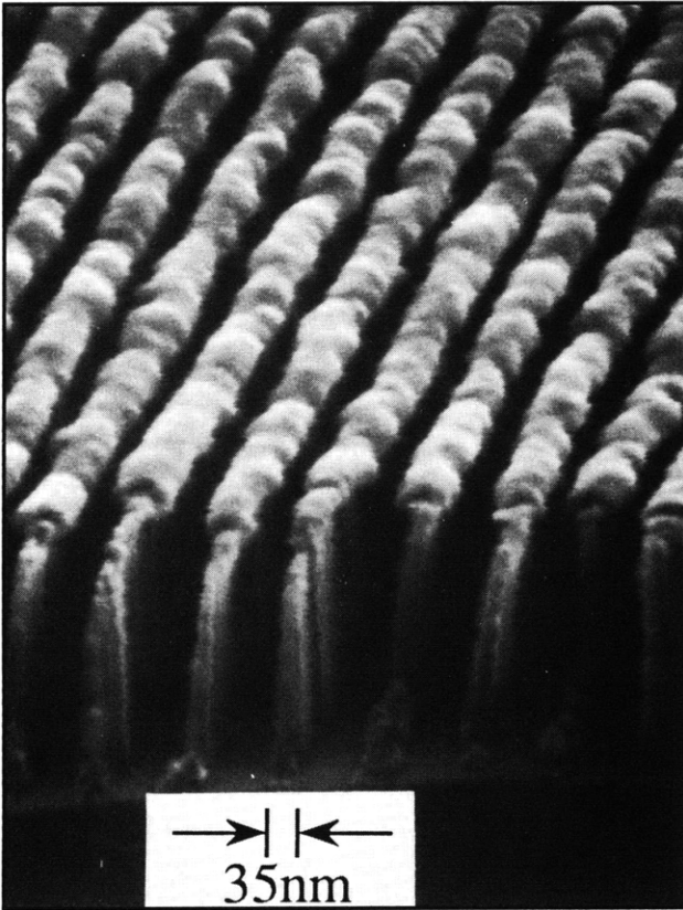
Figure 3. Scanning electron micrograph of 100 nm-period grating lines after exposure, shadow evaporation of nickel and reactive ion etching in an oxygen plasma.
