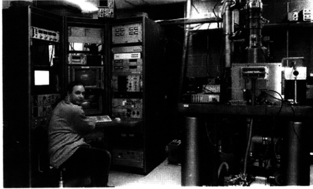
Figure 1. Photograph of the VS-PL scanning-electron-beam lithography system. The operator is Research Specialist Mark K. Mondol.
