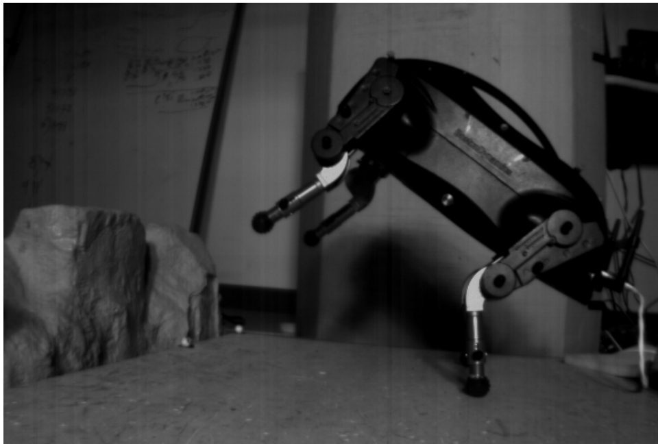
Figure 1-3: TOP: LittleDog robot walking on pegs. BOTTOM: LittleDog on hind legs.
