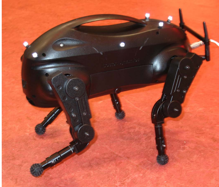
Figure 3-1: LittleDog Robot A picture of the LittleDog robot, executing the task of keeping its center of mass over the centroid of its support polygon, while moving the front-left foot in a fast Figure-8 trajectory. The robot has a 6 axis IMU and encoders at its 12 actuated joints as well as Vicon motion capture system for body position / orientation. The body weighs 1.8kg, and each leg weighs .25kg; The body is 20cm in length, while the upper arm is 8cm, and the lower arm is 10cm. ©2007 IEEE [Shkolnik and Tedrake, 2007].
