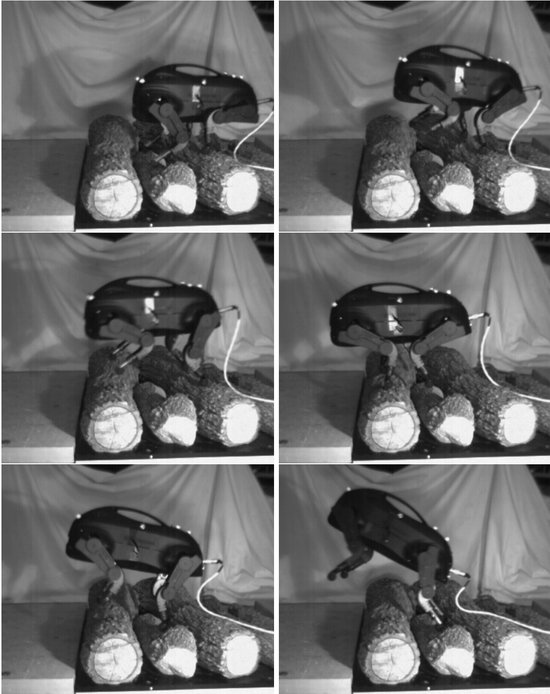
Figure 6-10: Bounding over logs with LittleDog
