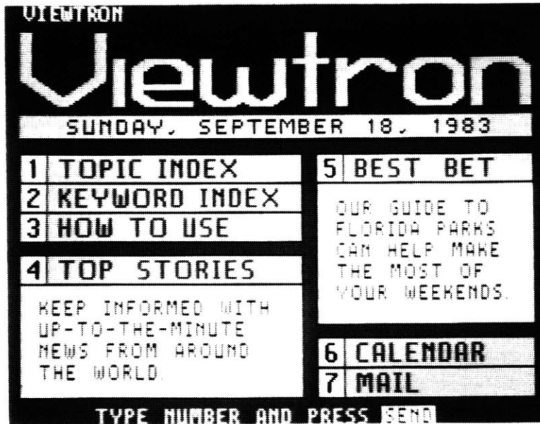
Figure 2-6: Videotex frame from Viewtron System
