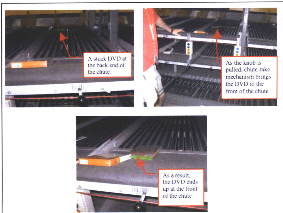
Figure 17: Chute Rake Operation
