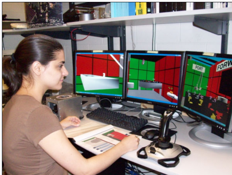
Figure 3.6: Experimental setup showing paper maps and typical camera views
