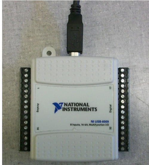
Figure 3.19: National Instruments DAQ card, model NI 6009.
