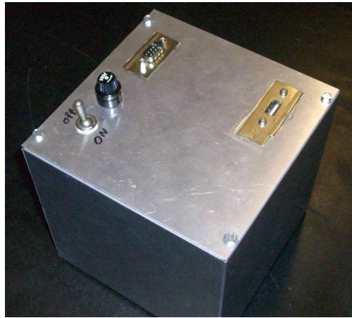
Figure 3.17: Metal housing of the thrust balance control box.
