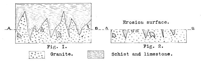
A rough diagramatic representation illustrating the very irregular contact between the schists and limestones and the granite, as it occurs in the district about L'Etang de Baxouillade, near the town of Ax-les-thermes in the Pyrenees.
