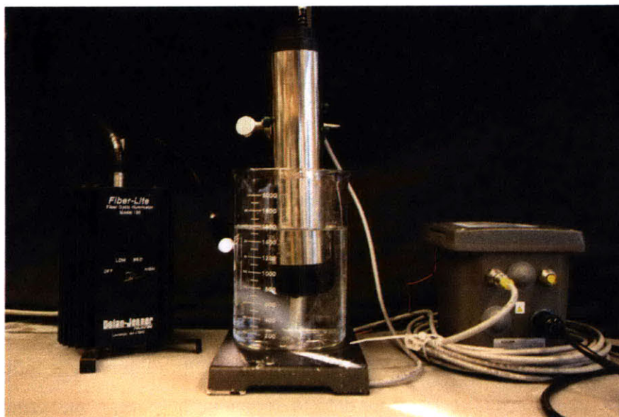
Figure 4-4: The Hach LDO dissolved oxygen probe, with the fiber lamp used to illuminate the sample.
