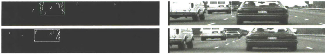
Figure 2-14: Example of locating targets at different disparity ranges. Top row: disparity range 7-9 at frame No.57 (Figure (2-7)). Bottom row: disparity range 7-9 at frame No.31. Left column: Edge closing operation result. Right column: segmentation result.
