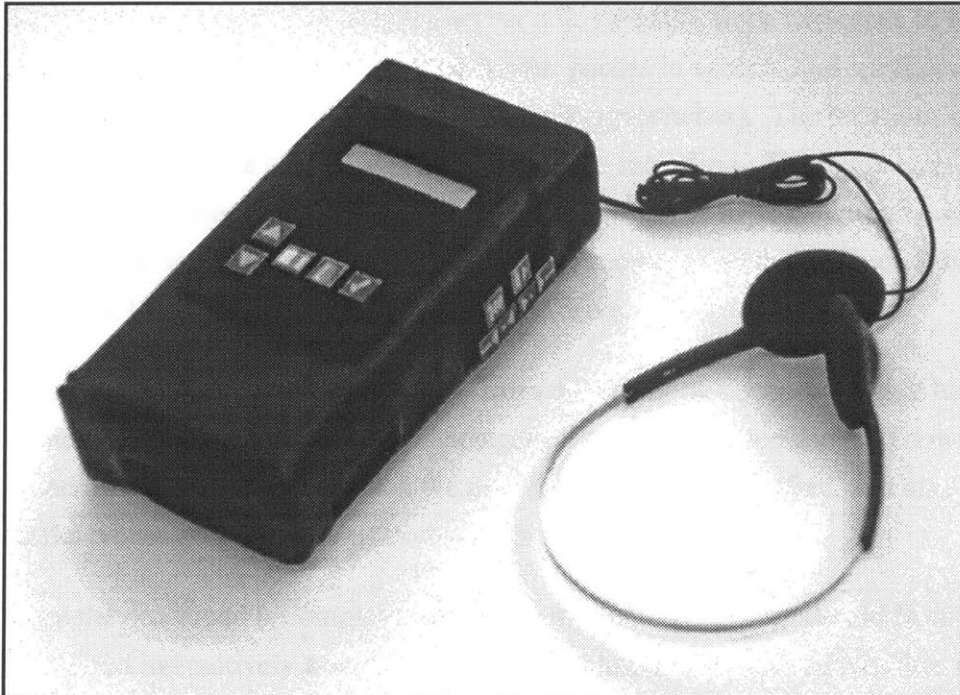
Figure 1: The NewsComm hand-held audio playback device with headphones. The top face houses a display and controls for selecting and managing recordings which have been downloaded into the hand-held's memory. The right side houses the navigation interface which can be controlled with the thumb while holding the device. The device can be connected to a central server to download personally selected digital audio recordings.
