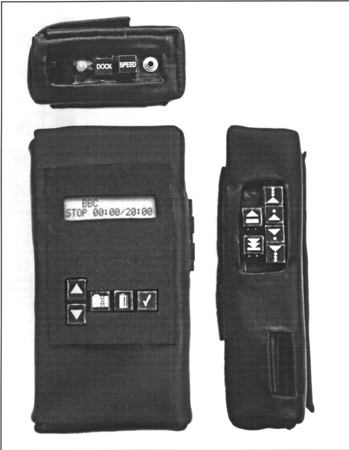
Figure 10b: Details of the top, front and right sides of the final hand-case which incorporates Version 5 of the interface design. The front panel houses the recording selection and management controls and a 2x16 character LCD screen, and the right side houses the navigation controls. The opening at the bottom of the right side provides access to the memory card eject slider. The case is made of soft leather and measures 7.5"(h) x 3.75"(w) x 2.0"(d).
