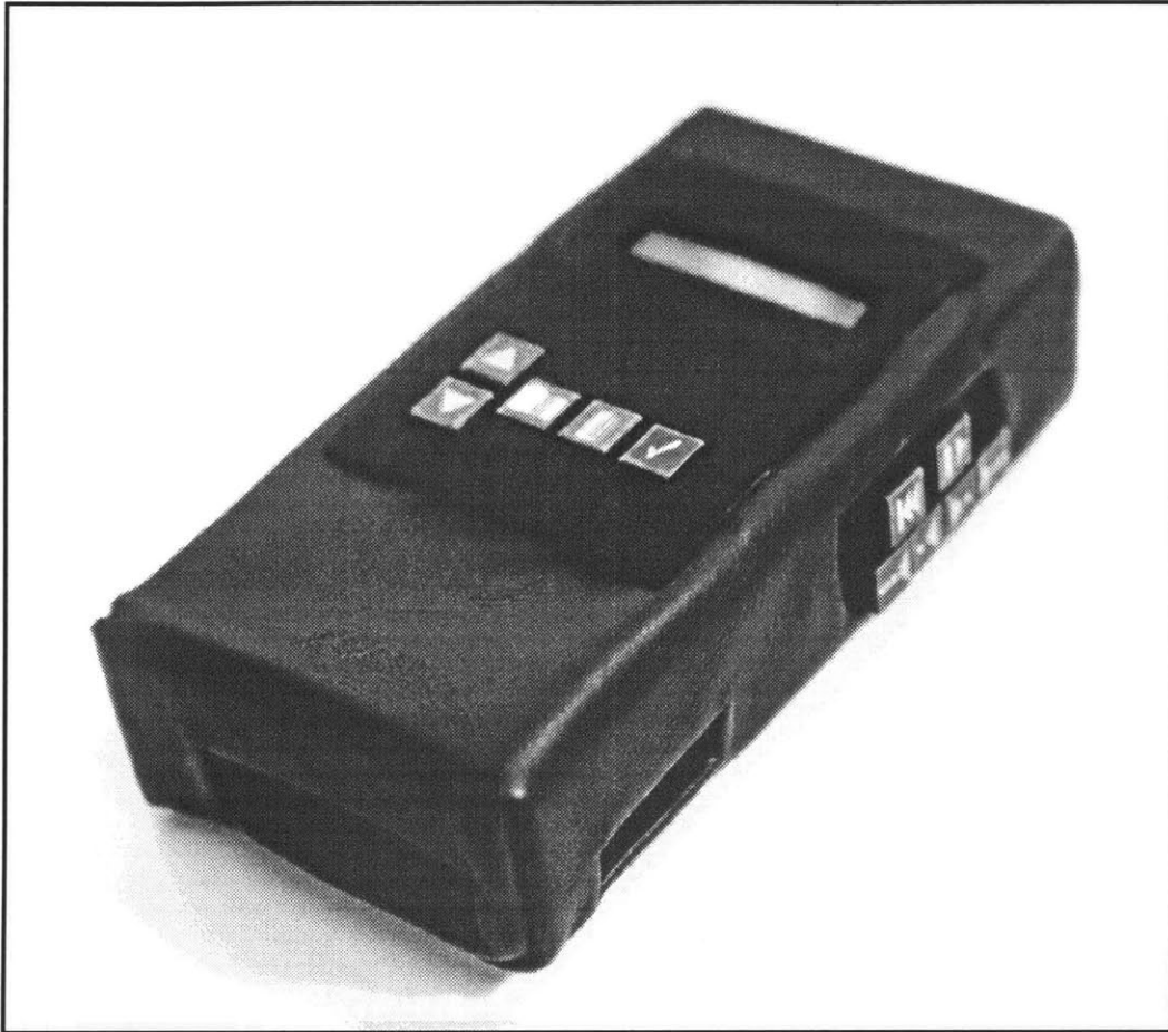
Figure 14: Photo of the final (version 3) hand-held. The case is made of soft black leather lined with cardboard supports from the inside. The HP95 is inside the case. The buttons are low profile tactile keyboard buttons. The screen is a 2 line by 16 character LCD module. The top panel (not in view) houses the main power switch, power indicator LED, headphone jack, and two buttons (the DOCK and SPEED buttons).
