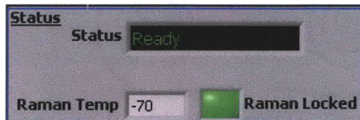
Figure 18 Raman CCD temperature locked to the target temperature
