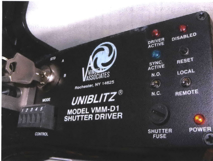
Figure 8 The shutter controller power switch and control settings
