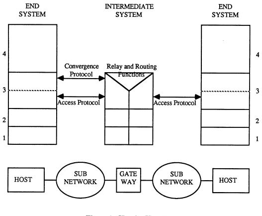
Figure 1: Hop-by-Hop Enhancement Source: Piscitello et al, Data Communications, May 1986, p. 122.
