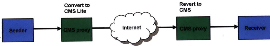
Figure 4-7: CMS Lite encode/decode
