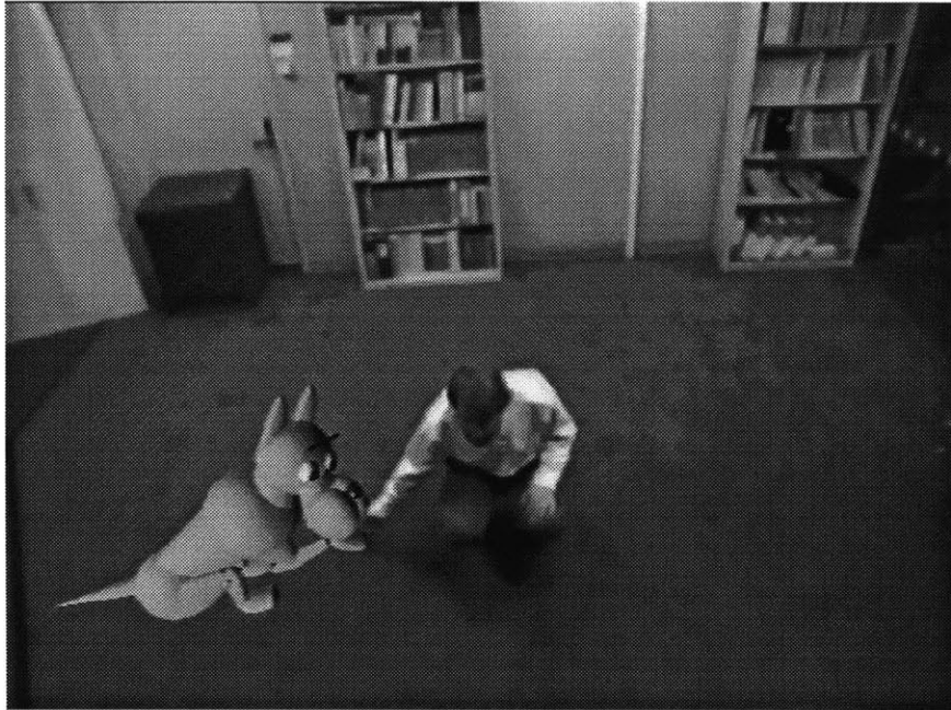
Figure 3-1: The composite image seen by an ALIVE user. Here the dog shakes hands because the user is sitting and holding out his hand.
